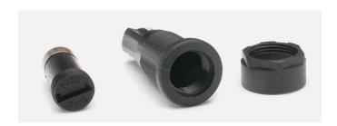
Low-profile panel mounting screwdriver release fuse carrier accommodating 5 x 20mm fuses. Hex nut fixing, depth behind panel 38mm. Rated 10A, 250V AC. Moulded insulating covers available.
