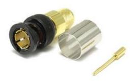
48-5069 COAX CONNS 10-005-W126-FD BNC 12G UHD Male cable, crimp, 75 ohm, black, group Z 48-5079 COAX CONNS 10-005-W126-FD BNC 12G UHD Male cable, crimp, 75 ohm, black, group Z (pack of 100)
