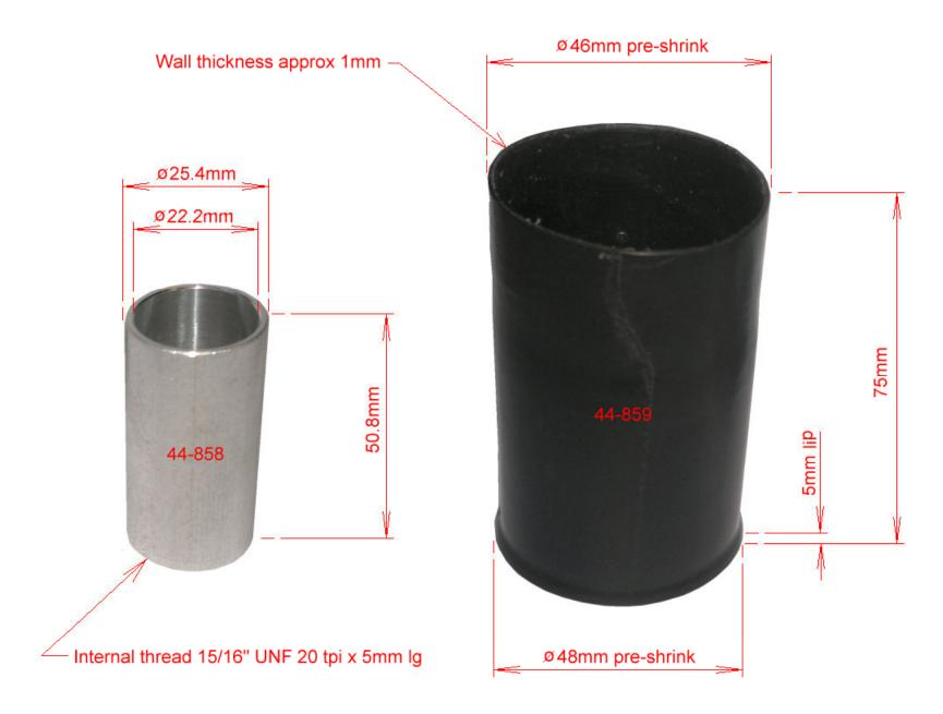
44-858 BAYONET-LOCK OB CONNECTOR 26 pin cable support ferrule 44-859 BAYONET-LOCK OB CONNECTOR 26 pin adhesive-lined heat shrink sleeve
