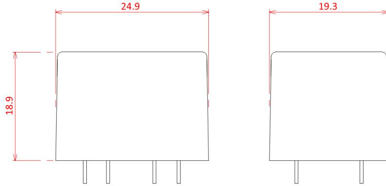
Suitable for microphone input stages optimised for medium source impedances ( $\sim 5\text{k}\Omega$ ), typical of medium Rbb bipolar transistors and operational amplifiers such as the NE5534. It can also be used for line level inputs when used in current mode active input circuits.
